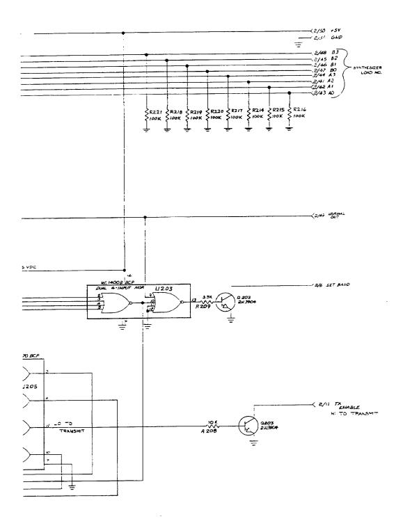
Fig. 2-6 Digital Control Board Schematic
