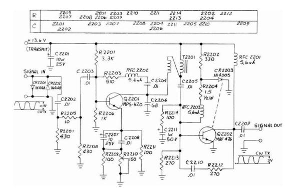
Fig. 2-40 Predriver Board #2 Pictorial & Schematic
