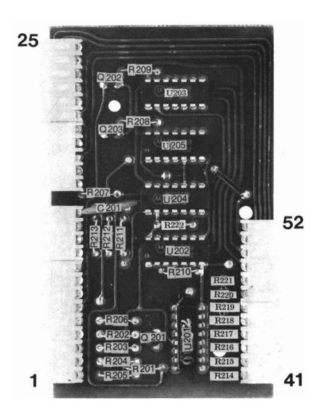
Fig. 2-5 Digital Control Board Pictorial
