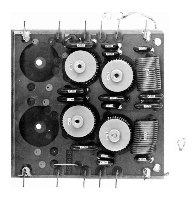
Fig. 2-33 Low Pass Filter Board Pictorial (Bands 1-4)
