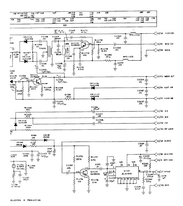
Fig. 2-24 2nd IF/Audio Board Schematic, Version 1
