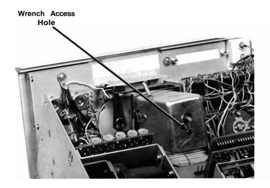
Fig. 2-43 PTO Torque Adjustment
