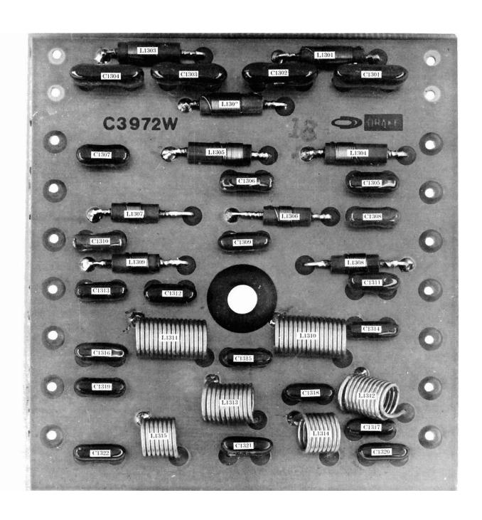
Fig. 2-30 High Pass Filter Parent Board Pictorial
