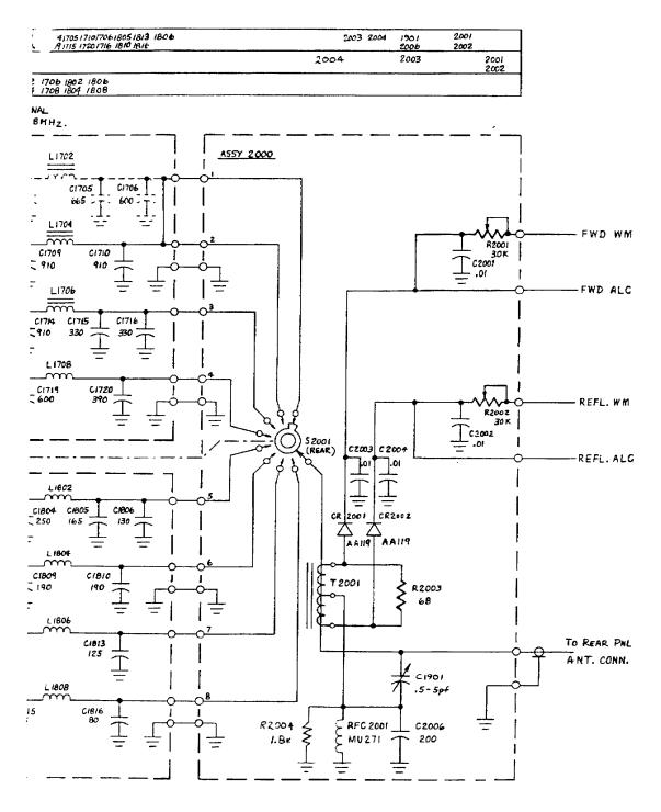
Fig. 2-36 Low Pass Filter Module Schematic
