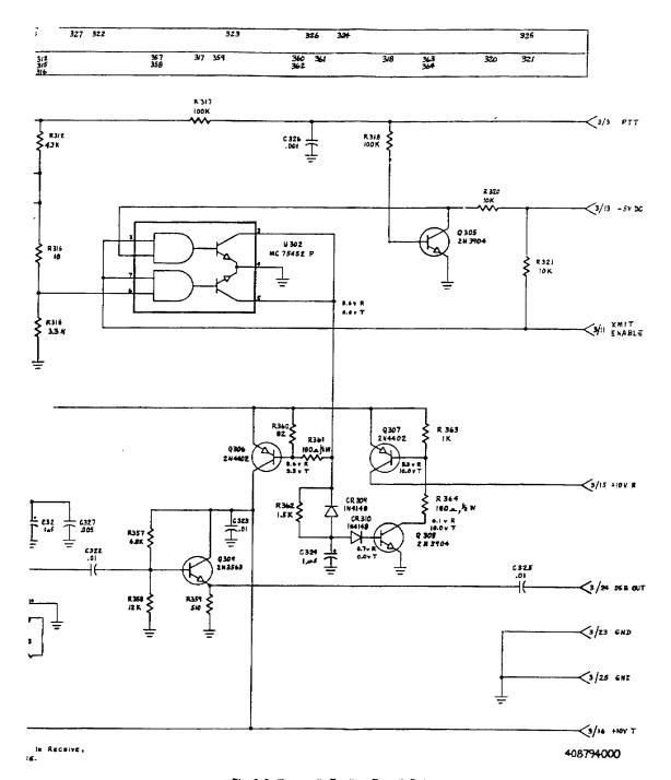
Fig. 2-8 Transmit Exciter Board Schematic
