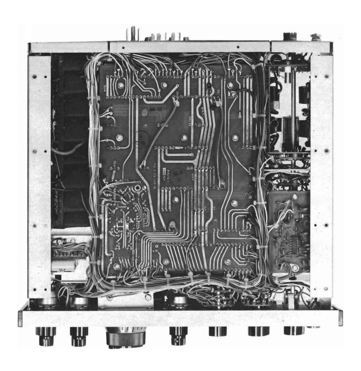
Fig. 2-3 Parent Board Pictorial (Bottom View)
