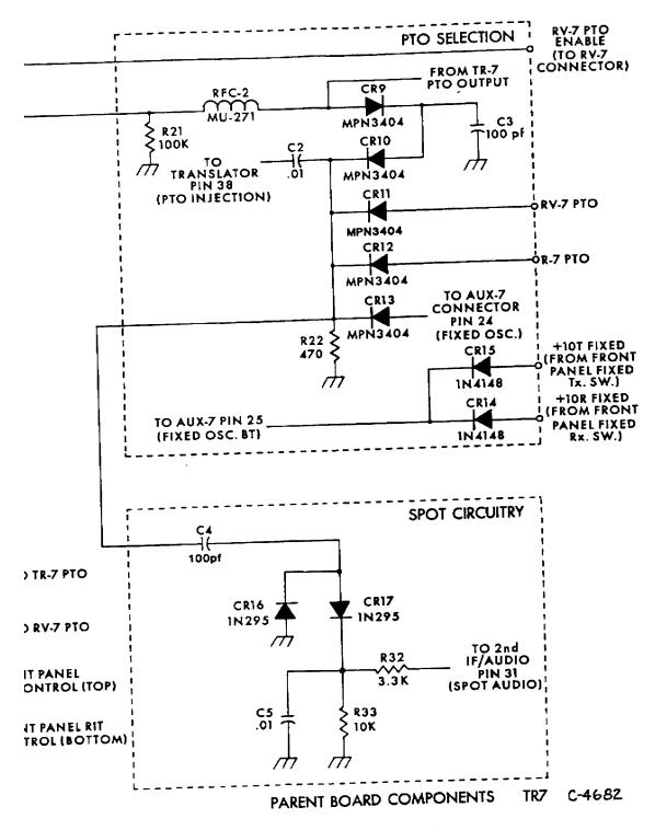
Fig. 2-4 RIT & PTO Switching Schematic
