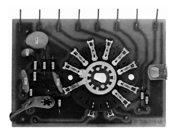
Fig. 2-31 High Pass Filter Switch Pictorial (Front & Rear)
