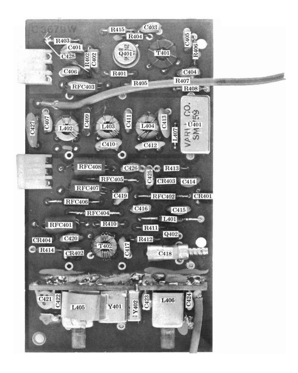
Fig. 2-9 Up-Converter Board Pictorial
