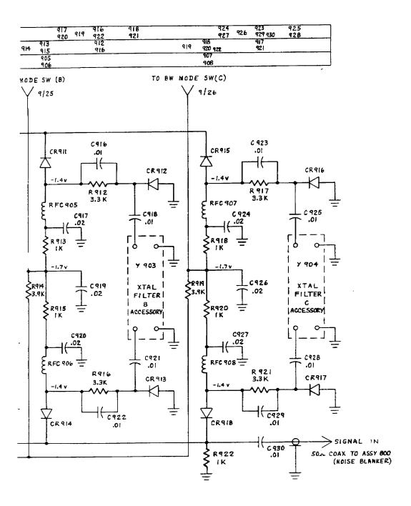
Fig. 2-20 IF Selectivity Board Schematic
