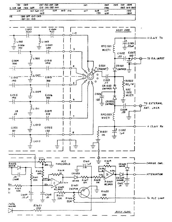
Fig. 2-32 High Pass Filter Module Schematic
