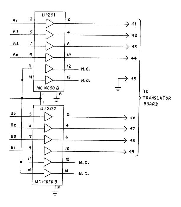
Fig. 2-28 Jumper Board Schematic
