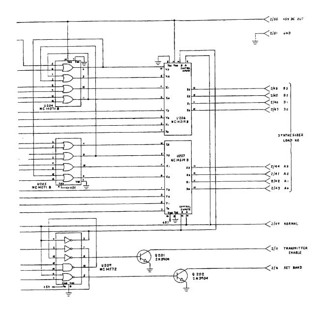
Fig. 2-6 Digital Control Board Schematic
