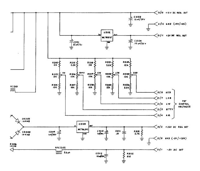
Fig. 2-38 Power Supply Board Schematic
