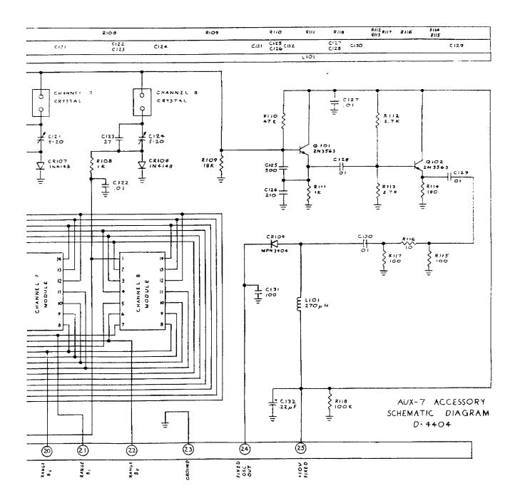
Fig. 4-5 AUX7 Board Schematic
