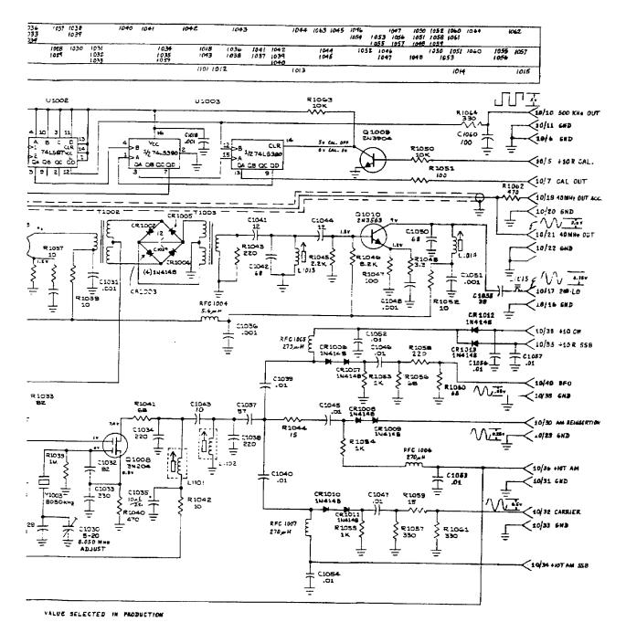
Fig. 2-22 PBT/Reference Board Schematic
