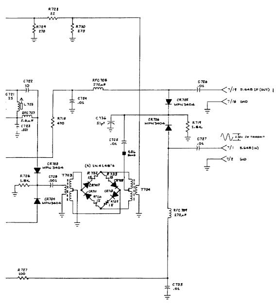
Fig. 2-16 2nd Mixer Board Schematic
