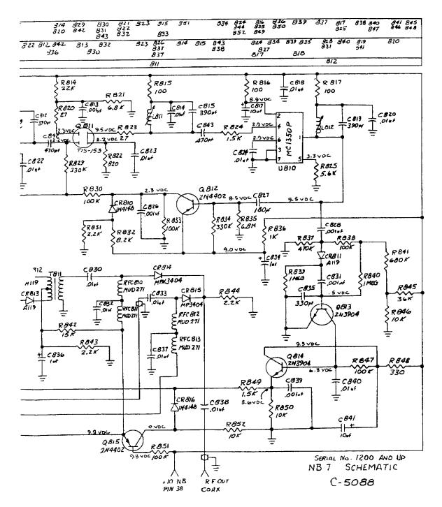
Fig. 4-9 NB-7 Board Schematic, Version 2
