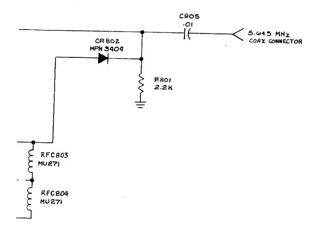
Fig. 2-18 IF Switching Board Schematic
