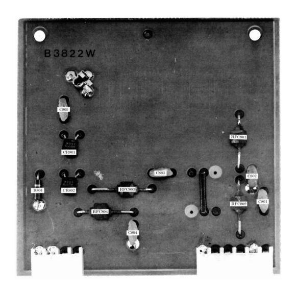
Fig. 2-17 IF Switching Board Pictorial
